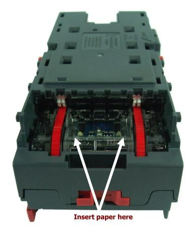
Repeat this procedure until all dust and debris has been removed from both belts. Finally, use a DRY lint free cloth to remove any excess moisture and refit the bezel. The bezel is refitted by pushing the bezel back onto the locating pins and sliding backwards until all six pins are engaged in the slots. The locking arms will then spring back and locate into the bezel.
